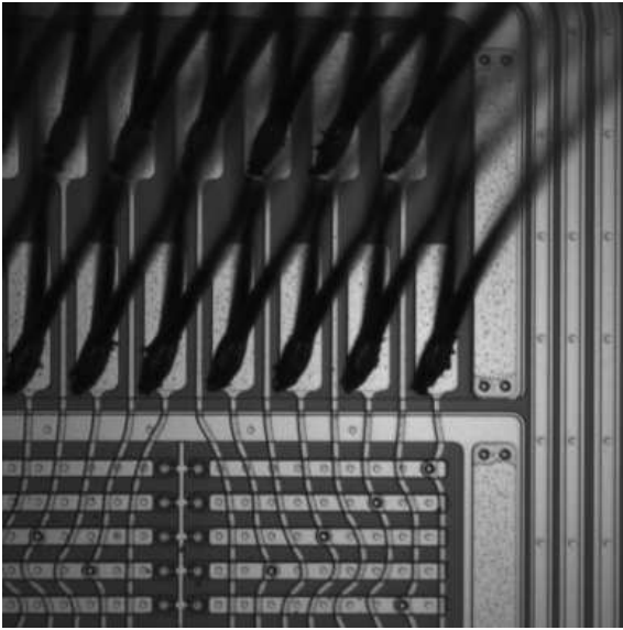
Figure 1: Sensor with interleaved readout pixels. Second metal layer provides 127 their interconnect and routing to the wire bond pad. Shuffling of readout chan- 128 nels minimises their cross-talk. 129
