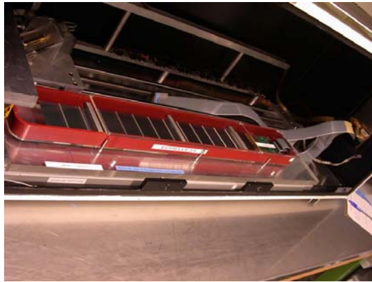
Figure 7. Example of the arrangement of the double-sided Si detectors on a ladder (a part of the tracker system of the AMS experiment).
