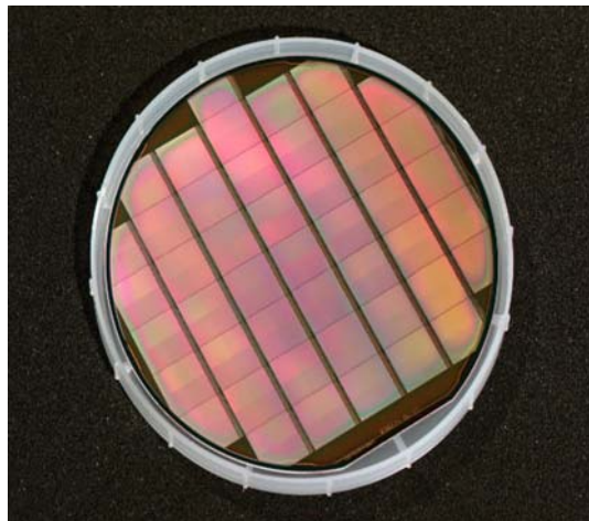
Figure 8. Prototypes of the MAPS detectors on 6" Si wafer.
