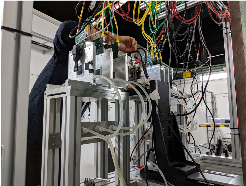
Figure 3.4: A photograph of the EUDET telescope at DESY from a test beam in December 2018. Here, the six telescope planes are clearly visible, with two RD53a modules situated between the two groups of three telescope planes.
