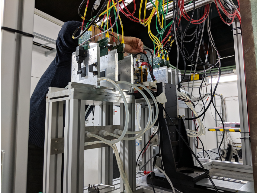
Figure 8.6: A photograph of the EUDET telescope at DESY from a test beam in December 2018. Here, the six telescope planes are clearly visible, with two RD53a modules situated between the two groups of three telescope planes.
