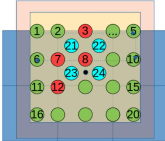
Figure 8.3: The different scan point positions used in the test beam. Scan point 8 represents the centre of the top middle ECAL module.
