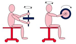
Change orientation of spinning wheel, volunteer rotates, see vector nature of angular momentum. E.g. wheel axis initially vertical, angular momentum vertical. Change to horizontal (volunteer must apply torque!) then volunteer's rotation ensures angular momentum of system (no external torque) conserved.
