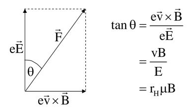
Here μ is mobility, with correction r<sub>H</sub> due to effects of B field. This causes displacement of hits:
