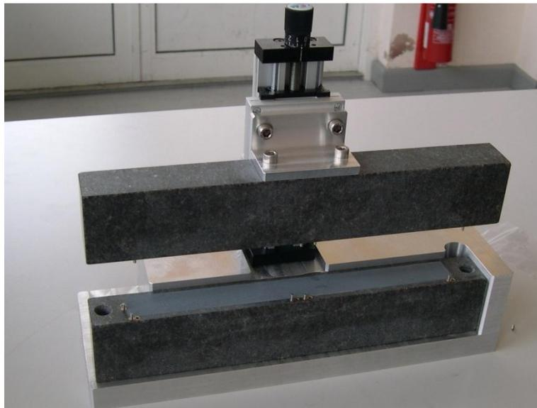
**Figure 28** A photograph of the new ladder-building fixtures showing the two granite flats with their ceramic foam inserts.
