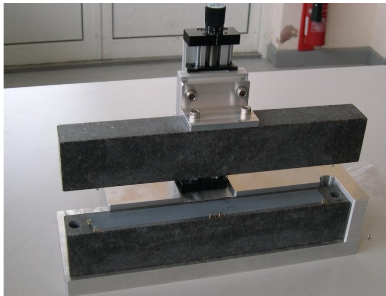
Figure 28 A photograph of the new ladder-building fixtures showing the two granite flats with their ceramic foam inserts.
