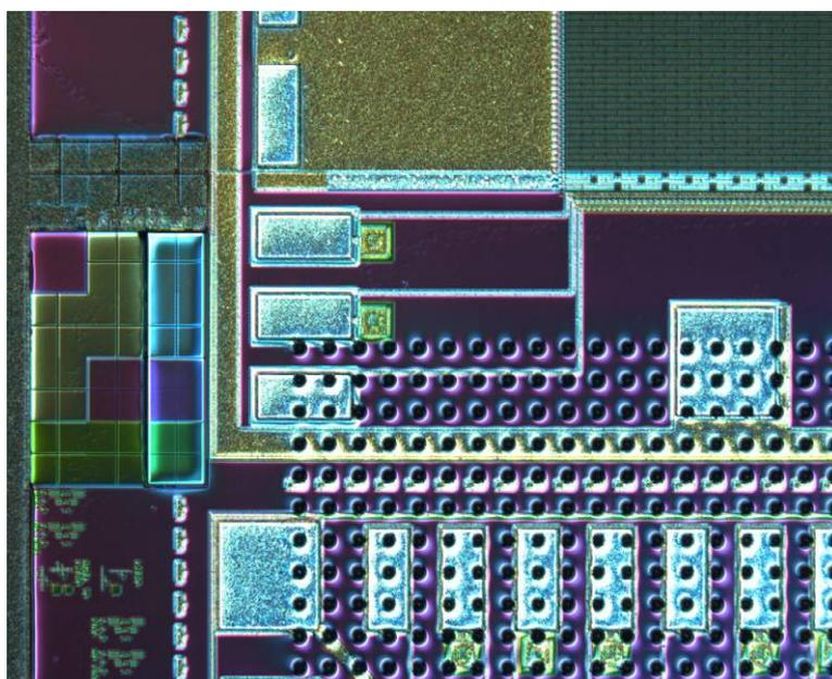
**Figure 17** Photograph of a CPC2 with deposited bump bonds and protective resist. The chip is ready for dicing
