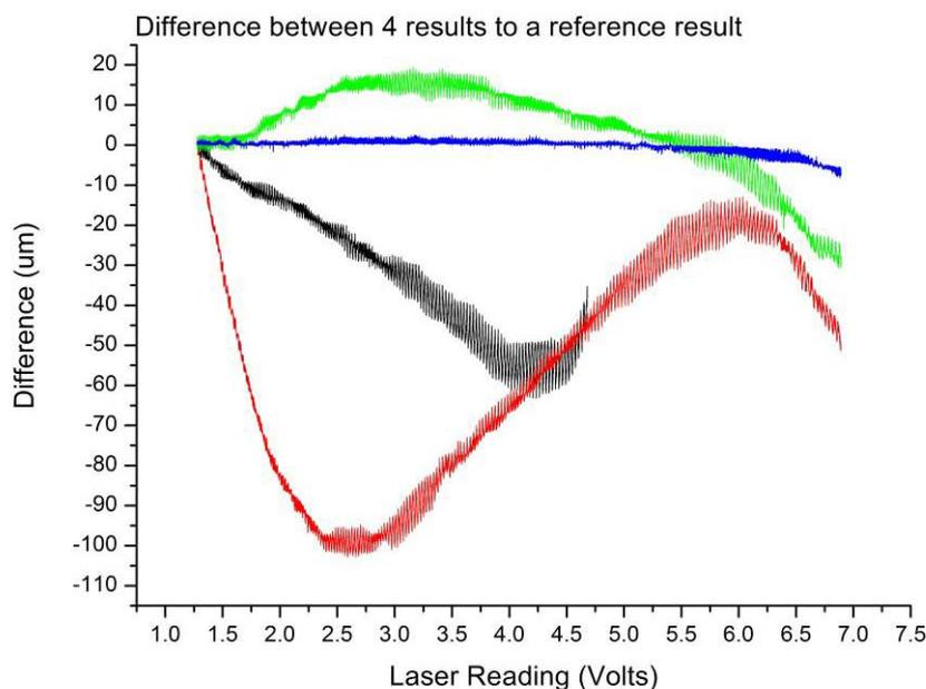
**Figure 20** LK-031 laser calibrations at various angles.
