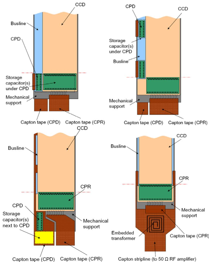
**Figure 15** Possible schemes for clock distribution to the CPD1 sensor: single CPD on CPC (top left); multiple CPD on CPC (top right); single CPD outside CPC (bottom left); transformer clock drive (bottom right).
