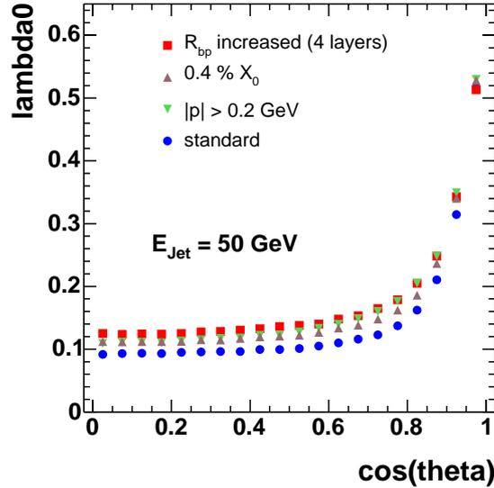
**Figure 4** Leakage rate as a function of polar angle for different detectors and reconstruction procedures.
