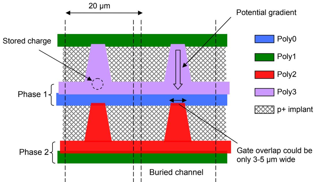
**Figure 6** Schematic design of open phase CCD
