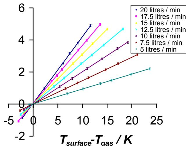
**Figure 22** Power extracted (in watts) from vertex detector model by gas as a function of flow rate and temperature difference.
