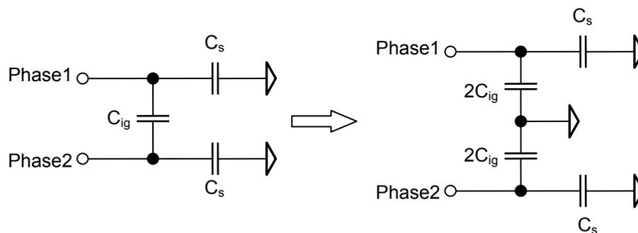
**Figure 5** Equivalent capacitance circuit for a 2-phase CCD
