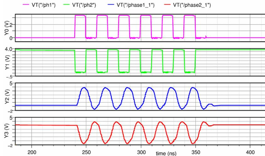
**Figure 11** CPD waveforms in Inverter Mode at 50 MHz.
