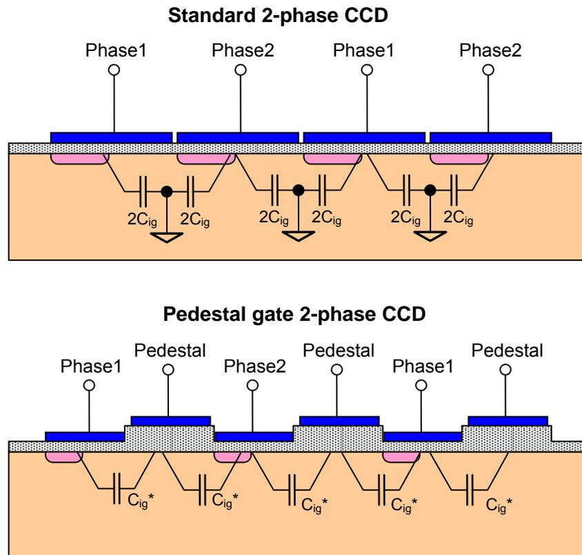
**Figure 7** Equivalent capacitance of the pedestal gate CCD. The capacitance to substrate is not taken into account.
