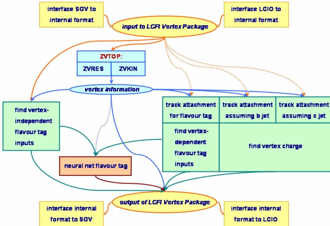
**Figure 1** Structure of the LCFI Vertex Package and flow of information between the different parts of the software.
