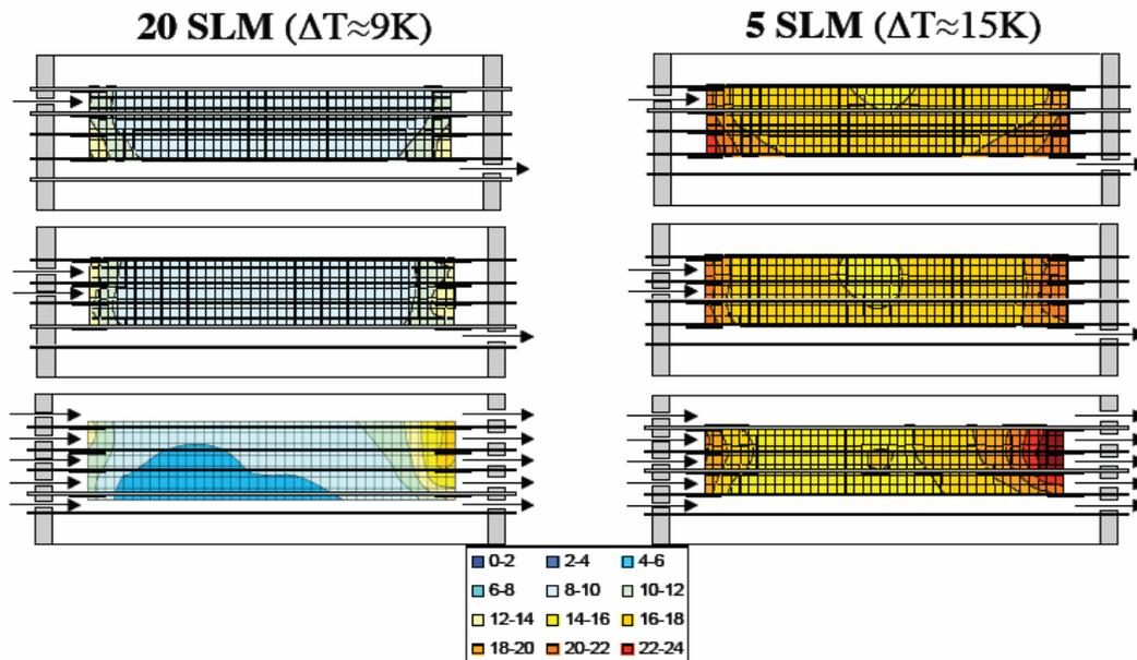
**Figure 23** Measured temperature distributions in the thermal vertex detector model for various inlet and outlet configurations.
