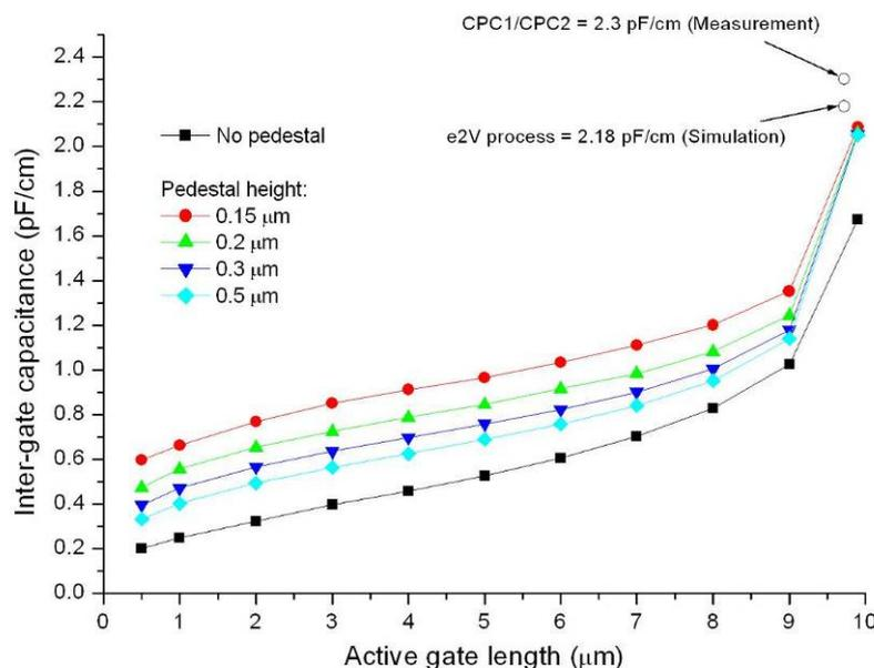
**Figure 8** The inter-gate capacitance as a function of the length and height of the pedestal gate. The pixel pitch is 20 μm.
