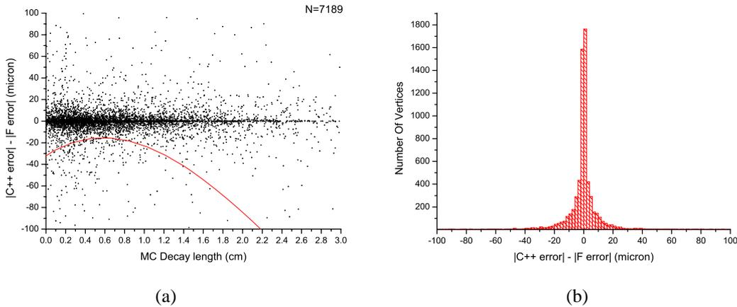
**Figure 3** Difference between the C++ and the FORTRAN deviation from MC in decay length, plotted as a function of decay length (a) and projected onto the y-axis (b). The red line in (a) shows a second order polynomial fit to the distribution.
