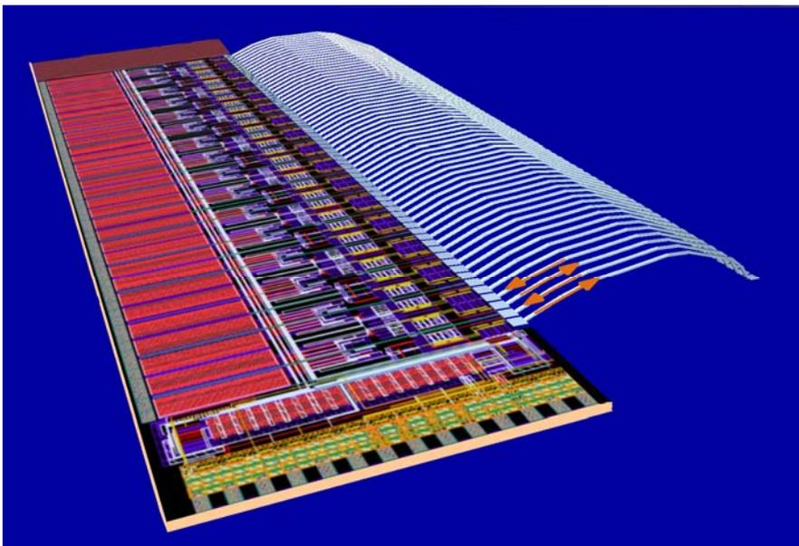
Figure 10 CPD1 layout with output bond wires
