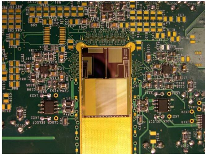
**Figure 13** MB 4.2 with CPC2-10 and two MAX5057 clock drivers.
