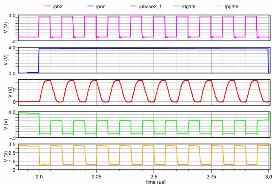
**Figure 12** CPD waveforms in Fast Mode at 10 MHz
