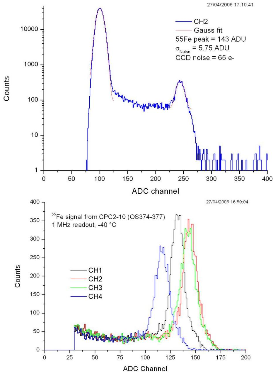
**Figure 16** The first <sup>55</sup>Fe spectrum obtained from one output of CPC2-10 at 1 MHz clock frequency (top), and the gain dispersion from 4 adjacent outputs (bottom).
