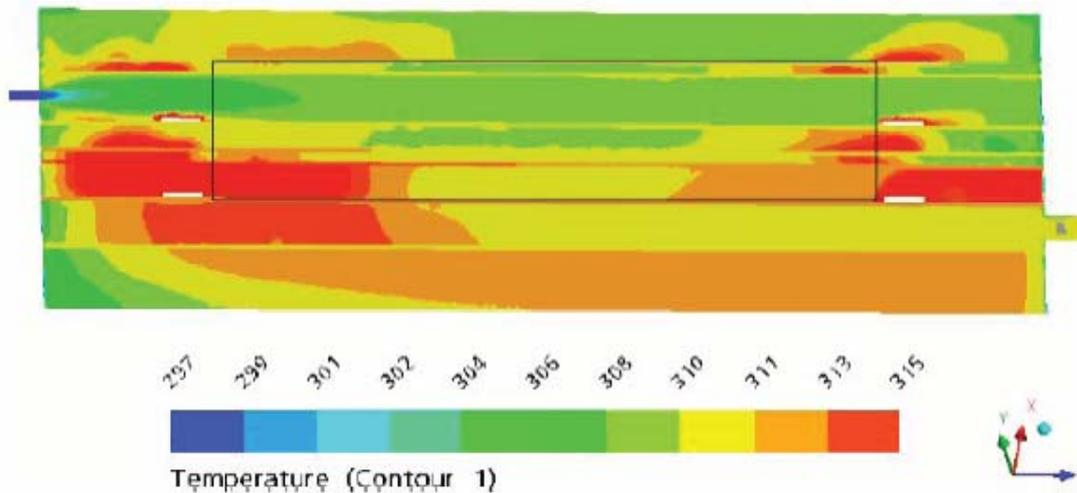
**Figure 24** CFD results for thermal model for a gas flow rate of 20 litres/minute.
