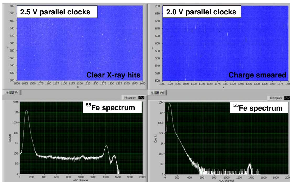
**Figure 9** Performance of DALSA FTF2416 at very low parallel clock amplitudes. Even at 2.5 V, the Mn  $K_{\alpha}$  and  $K_{\beta}$  lines are clearly resolved due to the very low readout noise. The serial clock frequency is 20 MHz.
