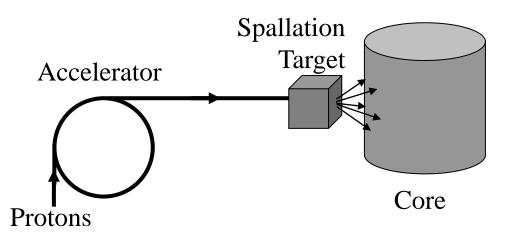
Run with k < 1 and use accelerator plus spallation target to supply extra neutrons.
