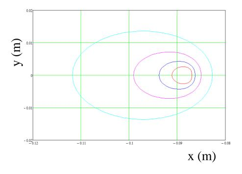
Focus poor as nominal position of focal plane is for object at infinity and "plane" should be curved!
