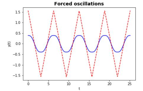
Motion including component due to a particular initial position and velocity.
