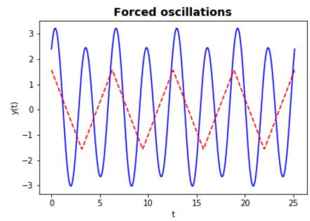
Friction would cause component due to initial motion to die out, leaving only that due to the force.
