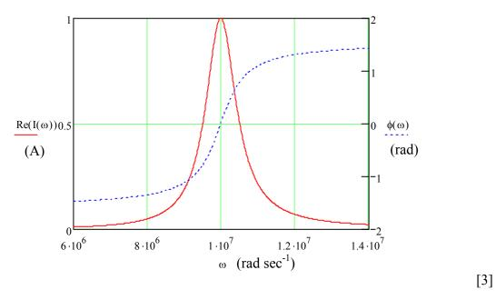
The current i has a maximum value of I =  $\mathcal{E}/R = 10/10 = 1$  A, [2] at the resonant frequency  $\omega = 1/\sqrt{LC} = 1/\sqrt{1 \times 10^{-9} \times 10 \times 10^{-6}} = 10^7$  rad sec<sup>-1</sup>. [2]
