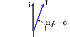
Now phasors for  $v_R$ ,  $v_C$  and  $v_L$ , with the phase relationships: i same as  $v_R$ ; i leads  $v_C$  by  $\pi/2$ ; i lags  $v_L$  by  $\pi/2$ .
