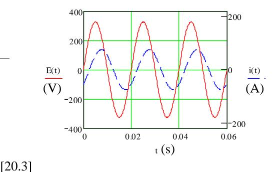
R = 3Ω, C = 1 mF, L = 0.1 mH so  $X_C = 3.18 \Omega$  and  $X_L = 0.031 \Omega$ .
