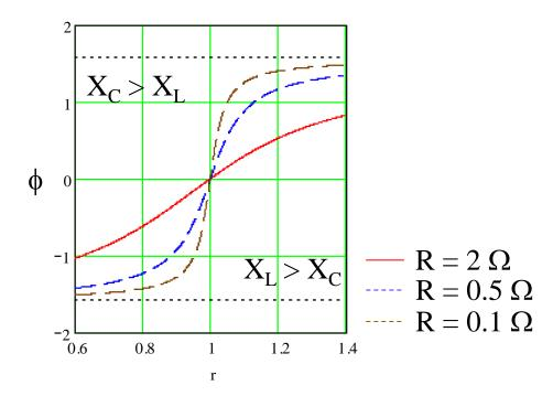
Phase increases from  $-\pi/2$ , through zero as frequency passes through resonance, to  $+\pi/2$ .
