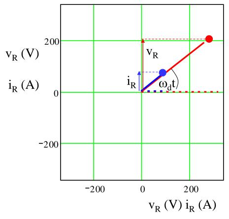
Allowing the phasors to rotate, we see how they describe the time variation of the current and voltage:
