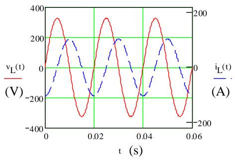
We see the current lags the voltage by π/2, (i.e. current reaches peak after voltage).
