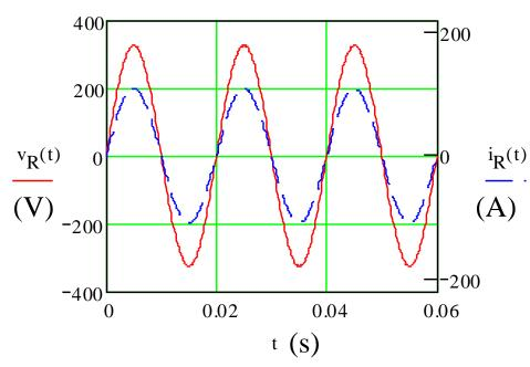
See the voltage and the current oscillate together, i.e. are in phase.
