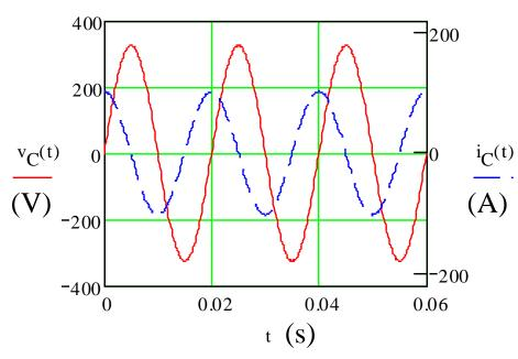
We see the current leads the voltage by π/2, (i.e. current reaches peak before voltage).
