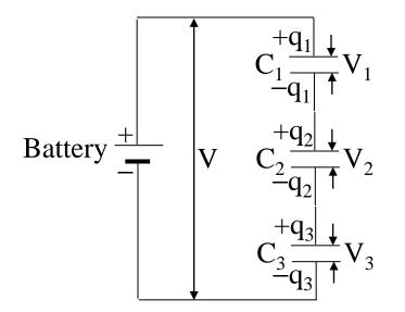
Now  $q_1 = q_2 = q_3 = q$ . (The battery "pushes" electrons onto the bottom plate of  $C_3$ , which repel the electrons in the top plate of  $C_3$ onto the bottom plate of  $C_2$ ...) The potential differences across each of the capacitors are:
