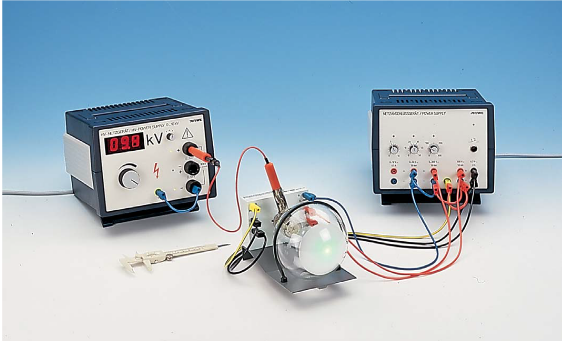
Figure 1: Electron diffraction apparatus showing faint green fluorescence rings generated by electrons hitting the screen.
