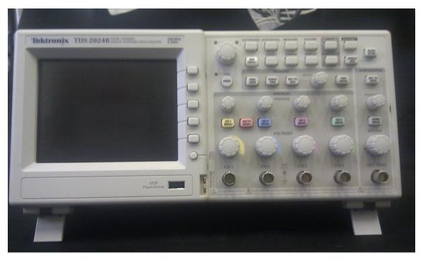
The signals generated by a pulse type detector can be viewed by an oscilloscope. The horizontal axis of the screen measures time and the vertical axis gives volts. An important characteristic of the oscilloscope is its bandwidth which determines the response of the scope to very high frequency signals. Modern oscilloscopes provide an analogue as well as a digital signal with bandwidths
