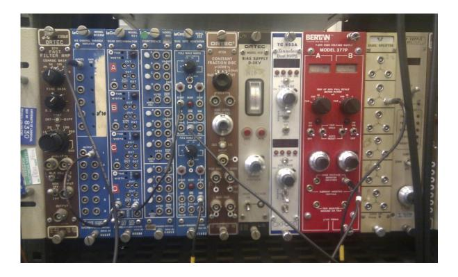
Most of the commercially available instruments that are used in high energy and nuclear physics conform to the standards of nuclear instrument modules (NIM). Any NIM module, for example a discriminator, power supply, amplifier etc., will fit in any NIM crate.
