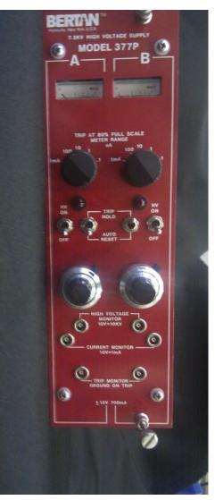
The high-voltage power supply (HVPS) provides a positive or negative voltage necessary for the operation of the detector. Most detectors need positive high voltage (HV).
