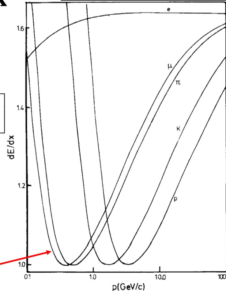
For different particle masses the spectra are shifted along  $p$ .
