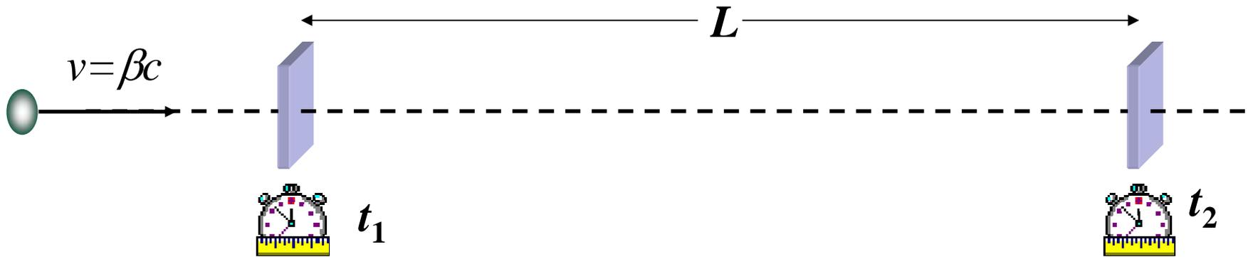
$$t_2 - t_1 = \Delta t = \frac{L}{\beta c} = \frac{L}{c} \sqrt{1 + \frac{m^2 c^4}{p^2 c^2}}$$
