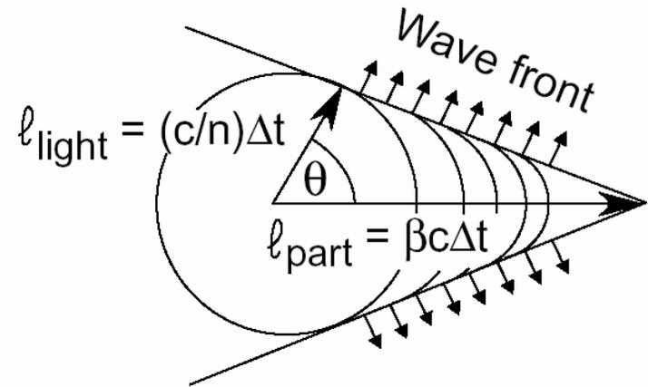
Huygens wavelets emitted all along the particles trajectory form a single wave front under an angle  $\theta_c$  w.r.t. the particle direction:
