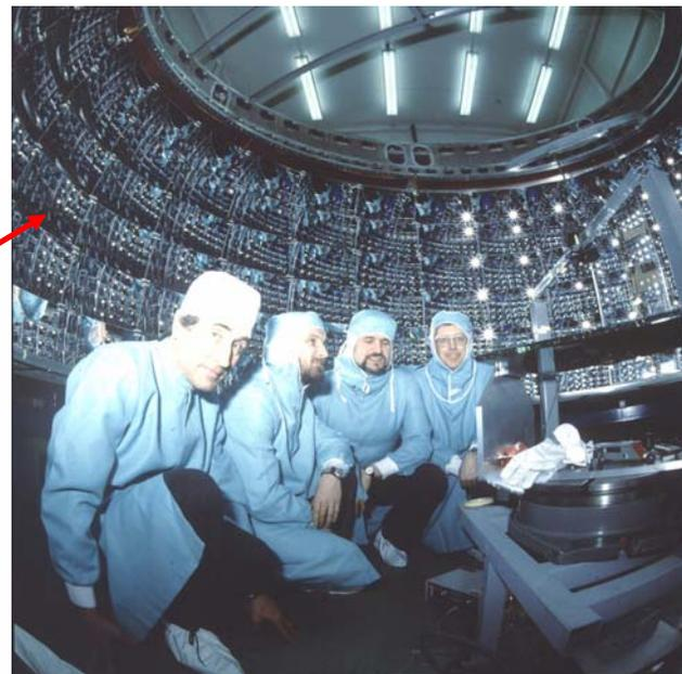
**Photon detector: TPC (with added photo-ionisation vapour, TMAE) with quartz windows and MWPC readout.**
