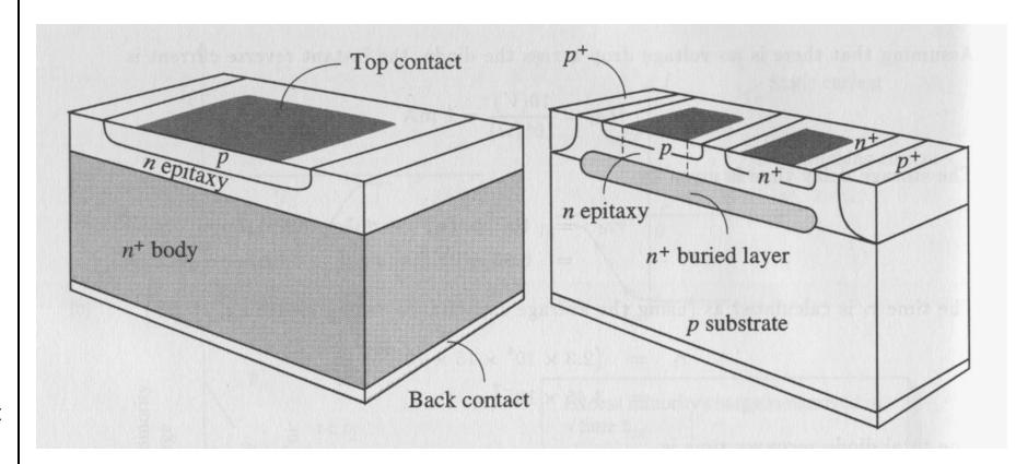
Cross section of a discrete p-n diode and a p-n diode in IC technology.
