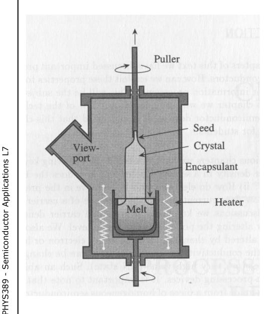
Silicon crystals have reached 30cm diameter and lengths approaching 100cm. Large size substrates ensure low-cost device production.
