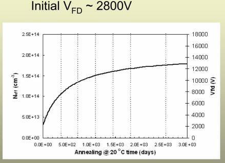
Predictions from RD48 parameters for Oxygen enriched devices (best scenario: after 7 RT annealing years the  $V_{fd}$  goes from ~2800V to ~12000 V!
