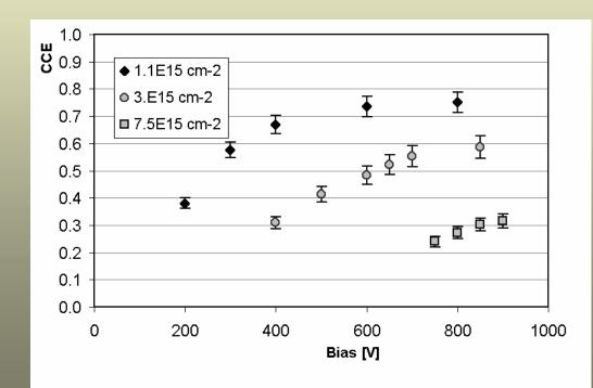
Degradation of the collected charge as a function of the irradiation fluence for n-in-p microstrip detectors. The applied voltages are 800, 800 and 900 volts for the three different irradiation fluences, respectively.
