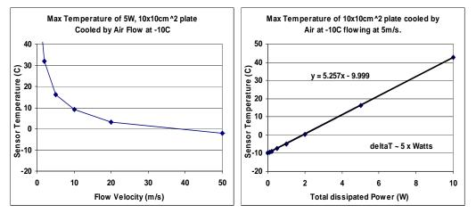
Calculating the exact cooling power required for higher energy running is not trivial.
