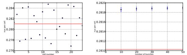
Figure 1: Simulated tune measurement using MIA in lattice without magnet or BPM errors. Left: Tune per cell, with 50 bunches per event. Right: Tune in cell 17, determined from events with different numbers of bunches. The red line shows the actual tune.
