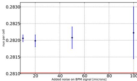
Figure 3: Effect of increasing BPM noise on simulated MIA tune measurement in cell 17 (50 bunches per event).
