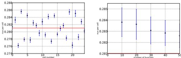
Figure 2: Effect of  $50 \mu\text{m}$  BPM noise on tune measurements. Left: All cells (50 bunches per event). Right: Cell 17.
