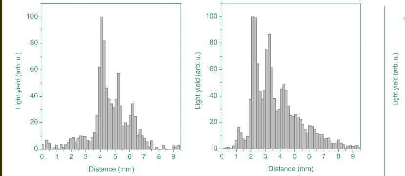
Intensity modulation caused by the pepper-pot grids for CsI:TI (left) and the SFOP (right). A resolution down to 0.3 mm was observed, but can be improved.
