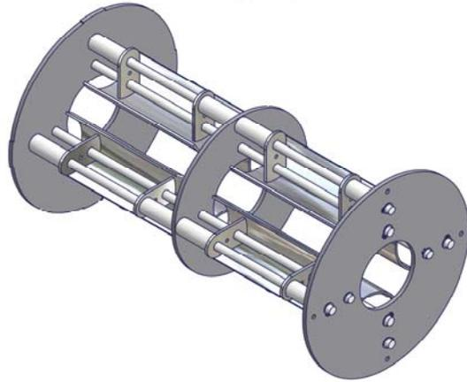
Figure 4: Mechanical design of the electrostatic quadrupole doublet.
