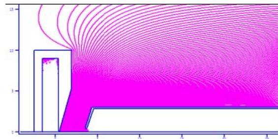
Figure 2: Extraction region behind the ion source with fields computed by POISSON.
