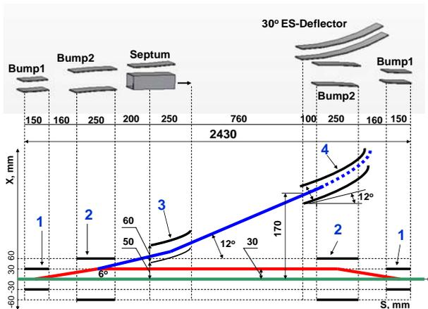
Fig. 7. Position of the USR beam extraction elements.
