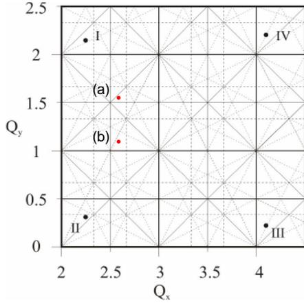
Figure 6. Tune diagram of the USR. (a) Betatron tune of the “round beam” operation mode ( $\nu_x=2.567$  and  $\nu_y=1.576$ ), (b) Betatron tune of the achromatic lattice used for short bunch operation mode ( $\nu_x=2.57$  and  $\nu_y=1.16$ ). The betatron tunes of the previous USR design based on  $90^\circ$  deflectors are indicated by I to IV.
