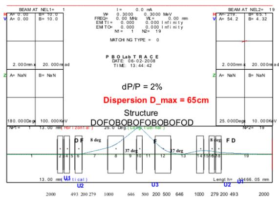
Figure 5. TRACE3D simulation of the central ray of the 300 keV pbar beam in one quarter of the USR.
