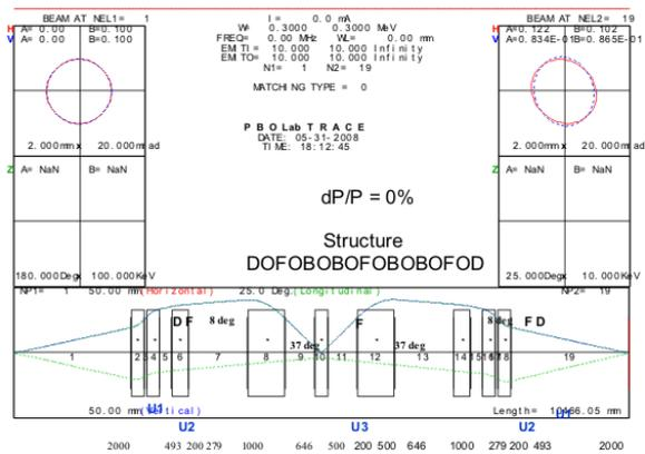
Figure 4. TRACE3D simulation of the 300 keV beam envelope in one quarter of the USR.
