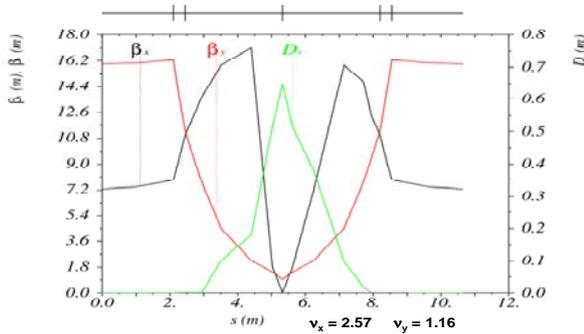
Figure 2. Beta-functions and dispersion of one ring quarter. A dispersion-free mode is used during short pulse operation. MAD-X simulation.
