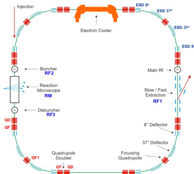
Figure 1: New layout of the USR.
