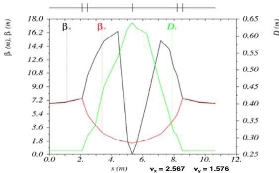
Figure 3. Beta-functions and dispersion in one USR cell for the round beam configuration.
