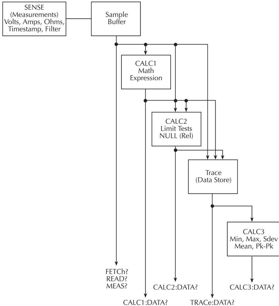
The SENSE block represents the basic measured readings of voltage, current, and resistance. If Filter is enabled, the readings will be filtered. The SENSE block also measures time for the timestamp.
