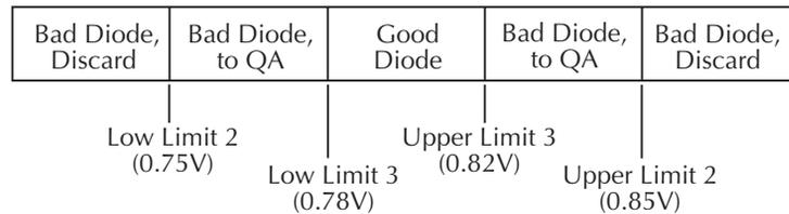
Table 12-3 summarizes the basic SCPI command sequence for performing a limit test for the diode breakdown described above, and Table 12-4 summarizes pass/fail parameters. Note that the test connections shown in Figure 10-8 can be used for this test.
