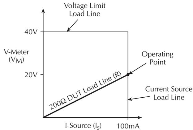
$$\begin{aligned} V_M &= I_S \cdot R \\ &= (100\text{mA}) (200\Omega) \\ &= 20\text{V} \end{aligned}$$
