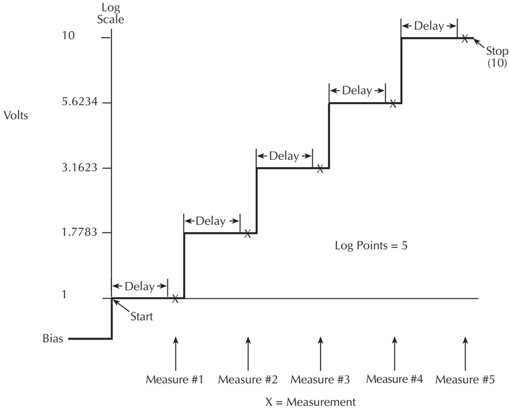
The programmable parameters for a log sweep include the start and stop levels and the number of measurement points for the sweep. The specified start, stop, and point parameters determine the logarithmic step size for the sweep. Step size for the sweep in [Figure 10-2](#) is calculated as follows:
