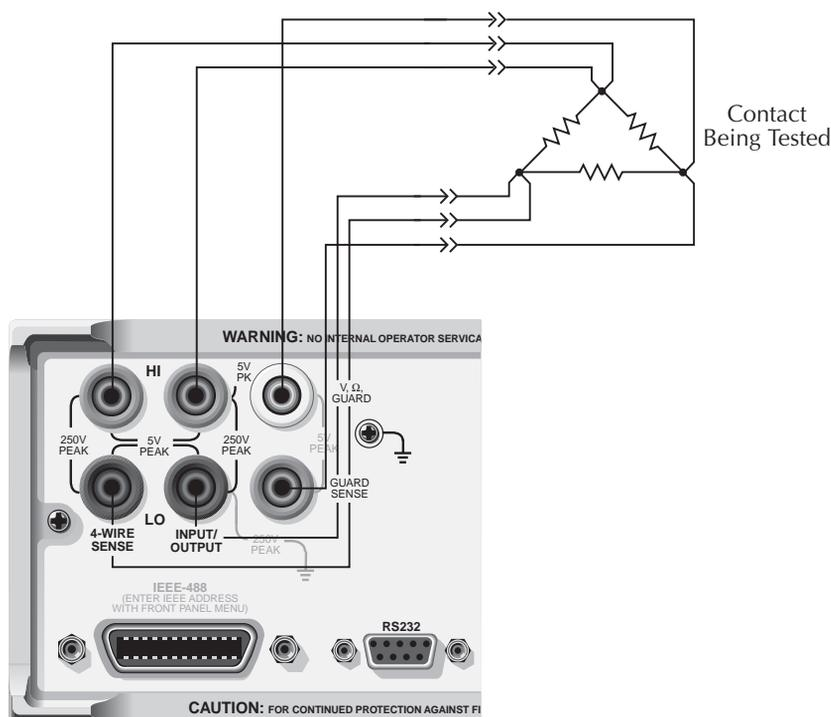
Note: Jumper V,  $\Omega$ , GUARD, and GUARD SENSE when using front panel terminals for contact check.
