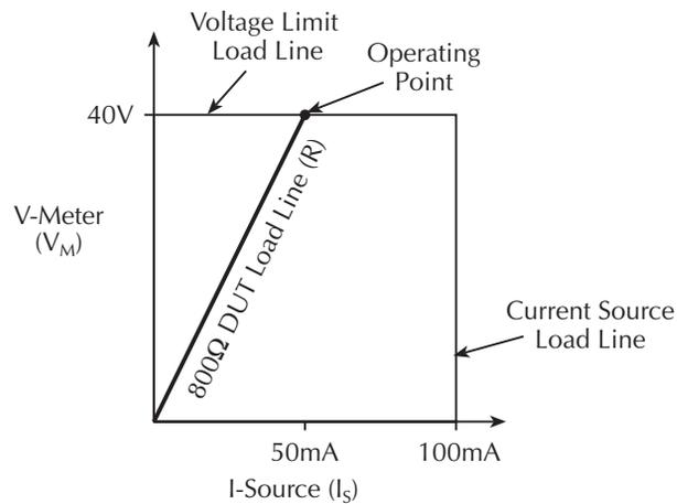
$$\begin{aligned} I_S &= V_M / R \\ &= 40\text{V} / 800\Omega \\ &= 50\text{mA} \end{aligned}$$
