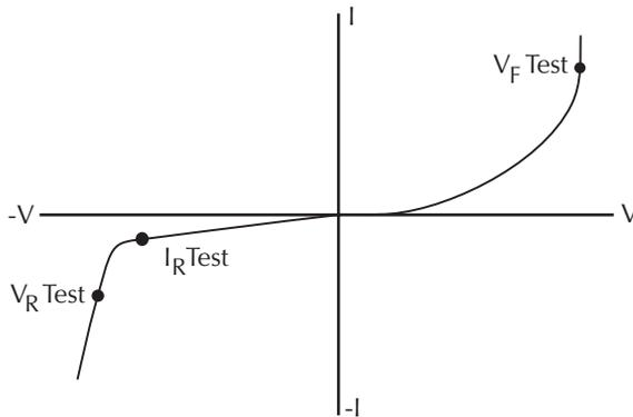
**Forward Voltage Test ( $V_F$ )** — This test involves sourcing a specified forward bias current within the normal operating range of the diode, then measuring the resulting voltage drop. To pass the test, the voltage must be within the specified minimum and maximum values.
