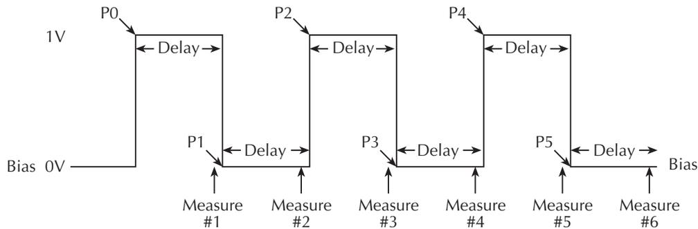
[Figure 10-4](#) shows a custom sweep example with different pulse widths. In this example, the first two points are configured with the same source value so that the duration of the first pulse is effectively doubled.
