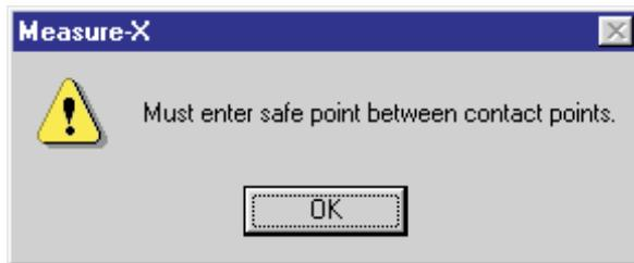
If either of the above messages is displayed, click **OK**, move the probe to a safe location, and press the Enter button on the joystick to record a safe point.
