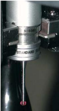
12. Lower or raise the probe sensor so that the top of the DSM is between the upper and lower lips of the port and the lower lip is centered in the DSM groove. This enables the DSM to be moved into the port smoothly.
