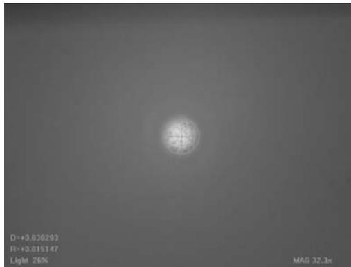
3. Display the top of the sphere in the Image window at high magnification.
