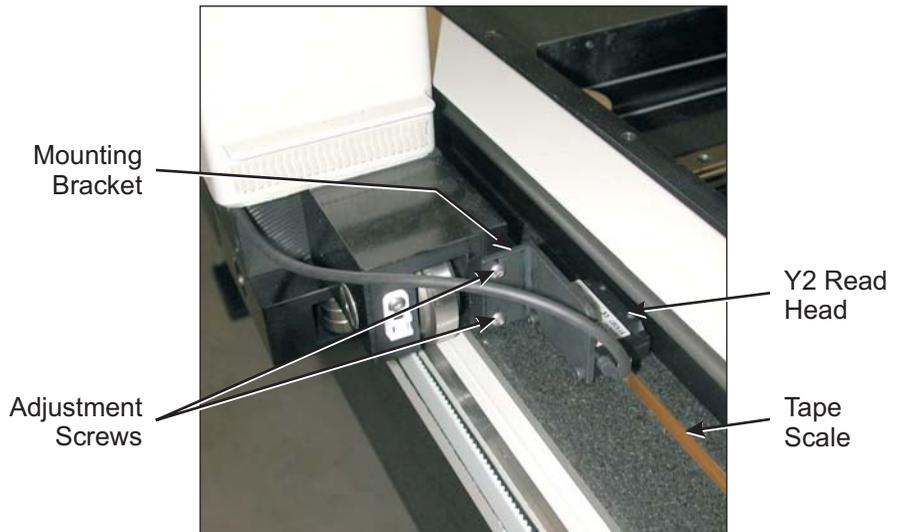
Figure 2-10. Installing the Y2 Read Head on the Left Side of the Machine
