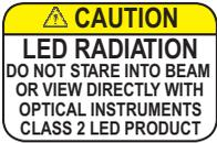
The SmartRing light is a Class 2 LED product. Do not stare into the illuminated LED beams or view them directly with optical instruments. Prolonged viewing of direct LED beams may be hazardous to the unprotected eye. However, momentary viewing (0.25 seconds) is not considered hazardous.
