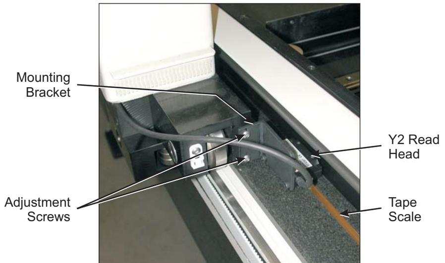
*Figure 2-17. Adjusting the Y2 Read Head Spacing*
