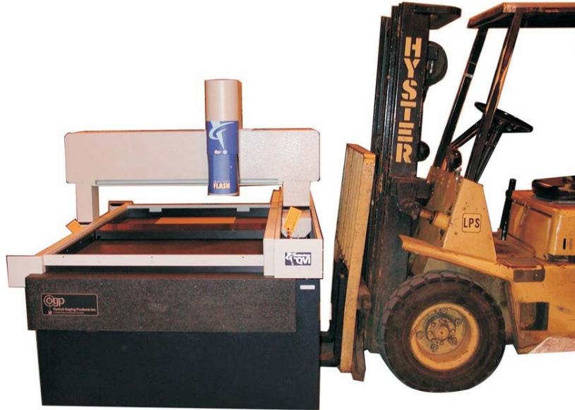
*Figure 2-4. Lifting the Machine*
