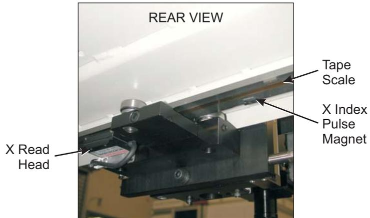
Figure 2-18. Location of the X Index Pulse Magnet
