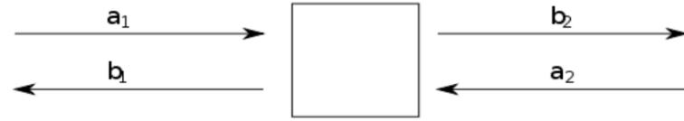
$$\begin{pmatrix} b_1 \\ b_2 \end{pmatrix} = \begin{pmatrix} S_{11} & S_{12} \\ S_{21} & S_{22} \end{pmatrix} \begin{pmatrix} a_1 \\ a_2 \end{pmatrix}$$
