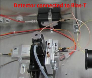
A small pad detector housing with test sample (FZ-p silicon diode) is included.
