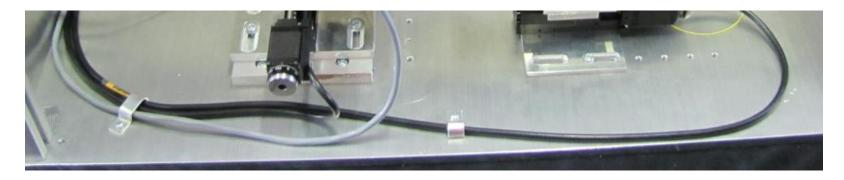
Once the stage cables are in position slide in the HV filter to the optimum position (no mechanical stress) and tighten the screw that fixes it to the back side
