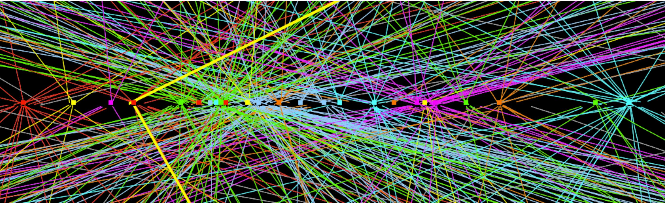
$Z \rightarrow \mu\mu$  candidate with 25 reconstructed vertices from the 2012 run. Only good quality tracks with  $p_T > 0.4 \text{ GeV}$  are shown
