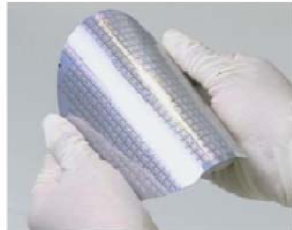
Wafer thinned to 50 microns (leti)
