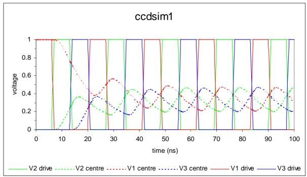
These results show that the CCD would not operate in the centre of the device at that particular frequency as the crossovers between the individual phases are not sufficiently defined.
