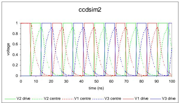
In this case, the voltage crossovers between the individual phases is sufficiently defined for the CCD to operate properly.
