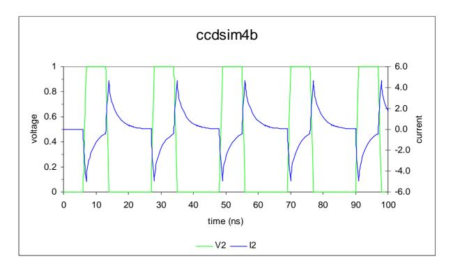
In the next example, the effect of adding some line inductance to the supplies to the CCD is modeled. A 200 pH inductance is placed in each phase between the voltage source and the feed to the corners of the CCD. The effect of the inductance upon the voltage waveform in each point of the CCD and upon the current drawn is shown below.
