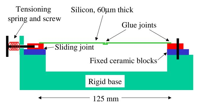
• For various tensions, repeatedly disturb, measure sagitta using ATLAS SmartScope.
