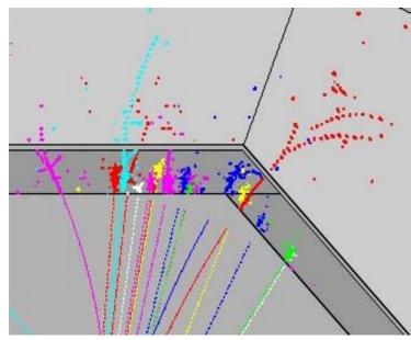
Use material with small Moliere radius and fine segmentation, readout 50 x 10<sup>6</sup> 1 x 1 cm<sup>2</sup> Si pads.
