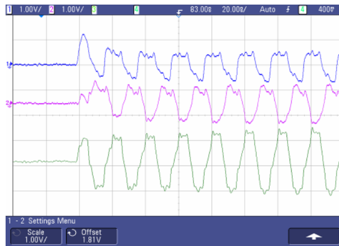
Figure 15 Oscilloscope trace of the two clock signals produced by the CPD1 and their difference.
