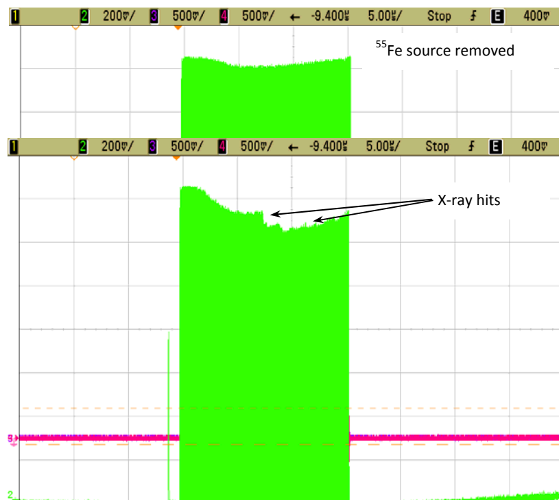
Figure 14 Oscilloscope traces of a discrete 2-stage CPC2-10 output at 45 MHz clock frequency with and without an ^{55}\text{Fe} source.
