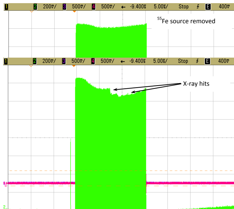
Figure 15 Oscilloscope traces of a discrete 2-stage CPC2-10 output at 45 MHz clock frequency with and without an ^{55}\text{Fe} source.
