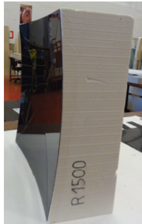
Figure 4.30: Mirror curved to radius 1.5 m.
