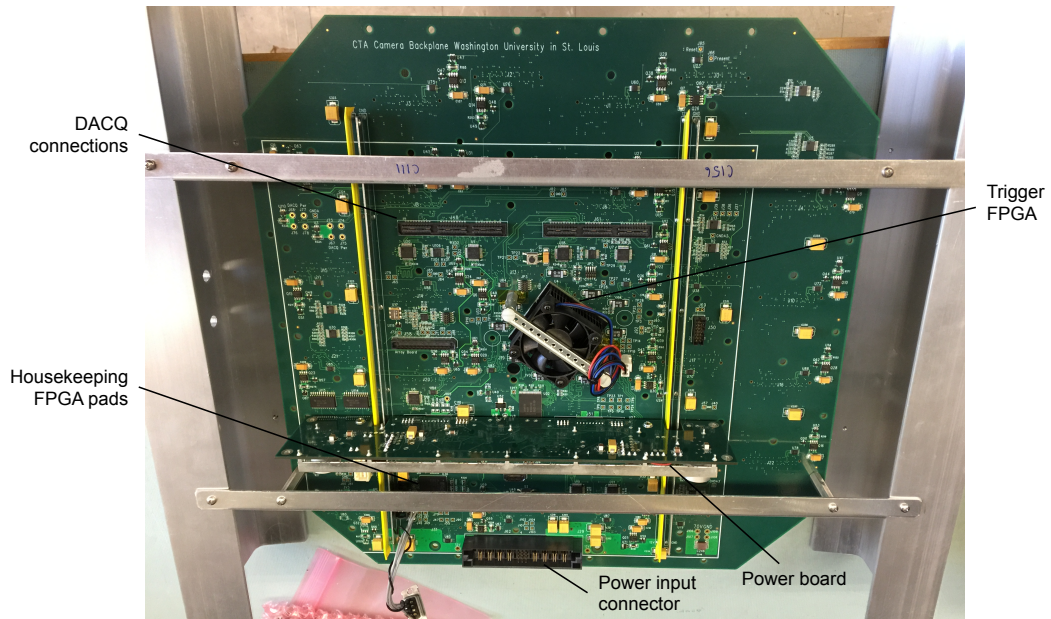
Figure 2.62 – The CHEC-M backplane with Xilinx Virtex 6 trigger FPGA and heat-sink mounted in the centre. Power for the backplane, DACQ and TARGET modules is routed from the power input connector to the power board mounted perpendicular to the backplane, where it is regulated and filtered. Connection to the DACQ boards is via the two large Samtec connectors located above the trigger FPGA.
