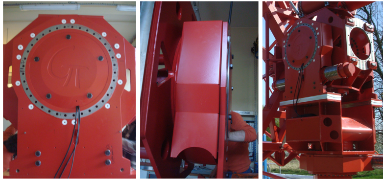
Figure 2.17 – Pictures of the lids covering the bearing. The rightmost picture shows the AAS mounted on the tower on the Meudon site.
