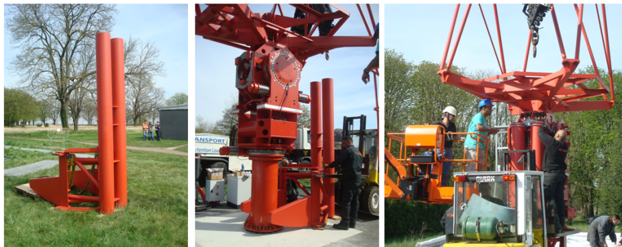
Figure 4.7 – The mounting of the counterweight on the prototype.
