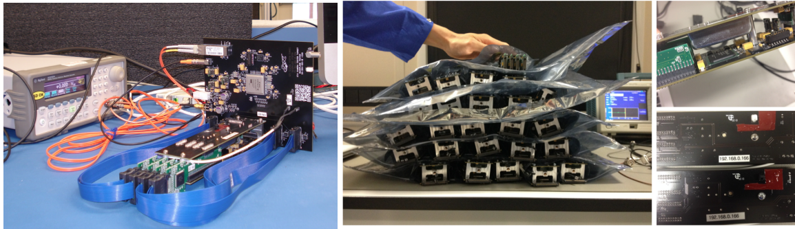
Figure 2.60 – Setup for acceptance testing of TARGET modules, using a custom made tester board PCB with signal generation and serial command/readout capabilities (left). The TARGET modules in Leicester (middle), some of which had duplicate IP addresses (bottom right) and missing heat sinks (top right) - both of which are now fixed.
