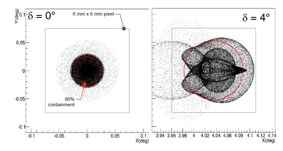
For field angles below about 5°, over 80% of the light from a point source at infinity (or at 10 km with refocusing) is contained in a 6 × 6 mm<sup>2</sup> pixel.
