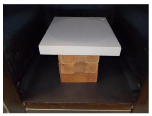
Level mould in oven and slump 4 mm thick glass sheet, 35 cm diameter, using carefully controlled temperature cycle.
