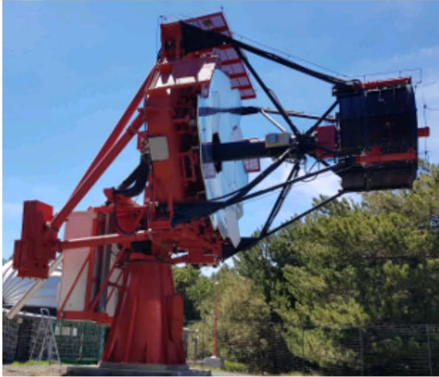
Figure 5.1: Photo of CHEC-S mounted on the ASTRI telescope structure at Serra La Nave Observatory, Sicily.
