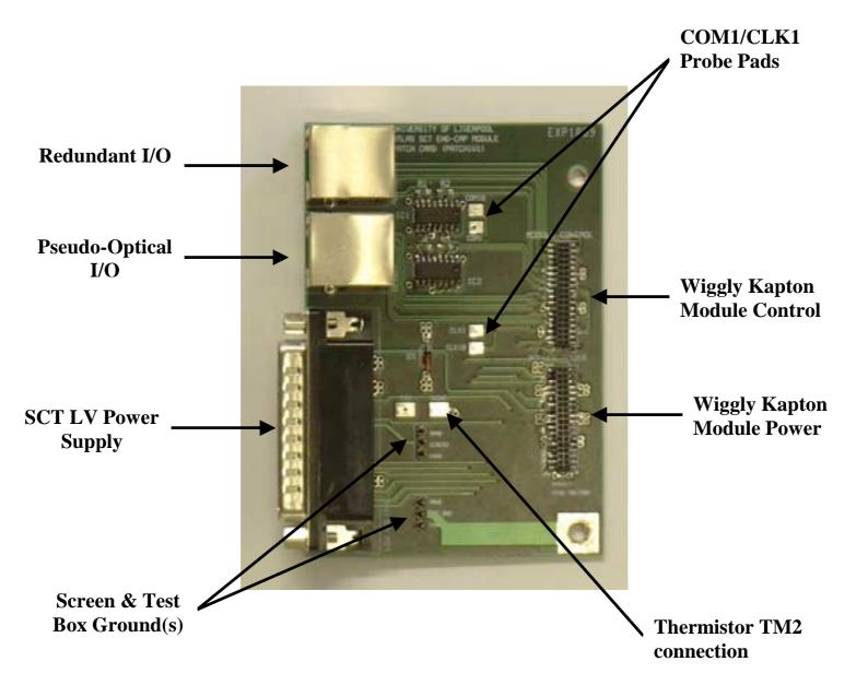
The Patch Card is designed to interface the VME Driver Board AERO (ATLAS Endcap ReadOut) to an Endcap Module using the Wiggly Kaptons. It provides the necessary connections for the module to be:
