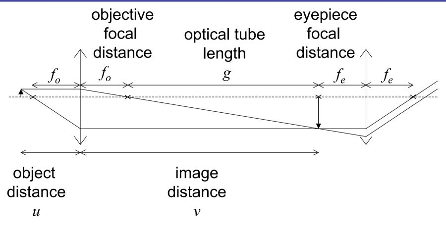
magnification of objective  $M_o = v/u = -g/f_o = -gF_o$  magnification of eyepiece:  $M_e = 25 \text{ cm}/f_e = 0.25F_e$
