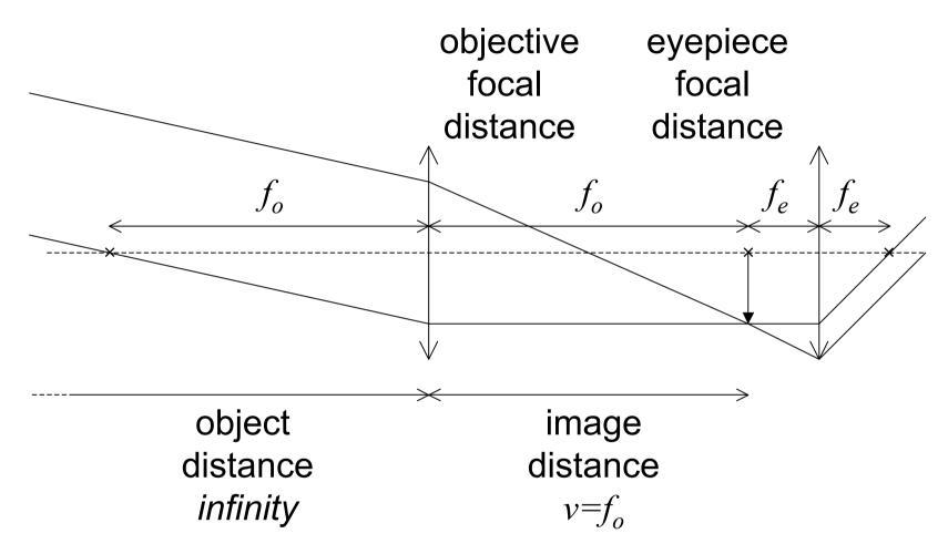
Magnification  $M = -f_o/f_e = -F_e/F_o$ Distance between the two lenses is  $f_o + f_e$
