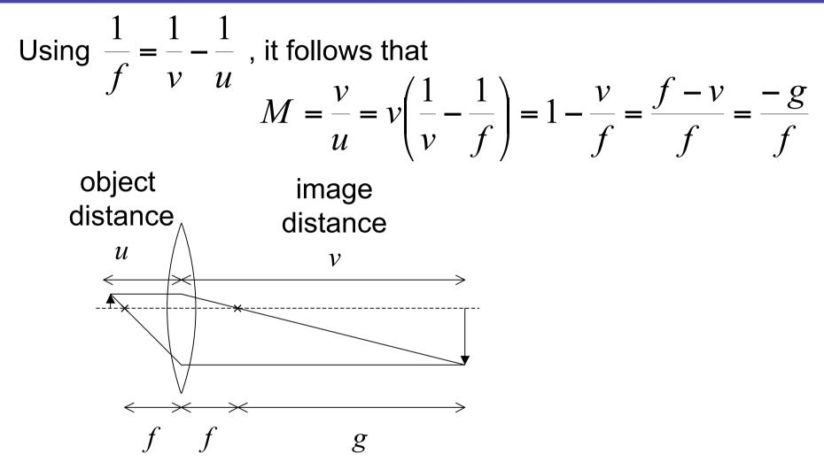
Magnification is the ratio of the distance g from the second focal point to the image and the focal distance f of the lens
