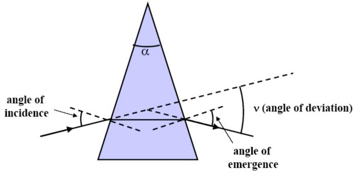
Smallest angle of deviation occurs in the above case, where the ray passes symmetrically through the prism.
