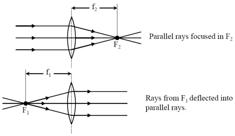
In general focal length  $f_1$  is equal to focal length  $f_2$  (but opposite sign). (not if medium on one side is different from that on the other side. E.g. contact lens.)
