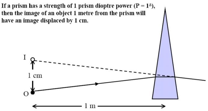
So a displacement of 3 cm at  $\frac{1}{2}$  a metre would give a dioptre of  $P = 6^{\Delta}$
