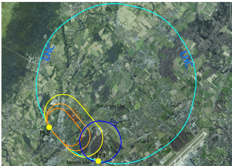
Figure 10.49: Racetrack options proposed for LHeC at Point 2 of the LHC. The color coding illustrated different options with 1/3 , 1/4 and 1/5 of the LHC circumference, resulting in different electron beam energies.
