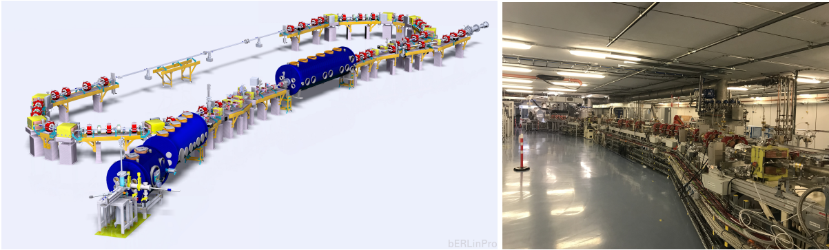
Fig. 6.2: Left: The layout of bERLinPro, which is essentially complete apart from the 1.3 GHz linac module and the upgraded 100 mA gun, the main hardware elements of the Roadmap for bERLinPro; Right: View from the dump position of the injector (at the back) and first racetrack part (June 2021).
