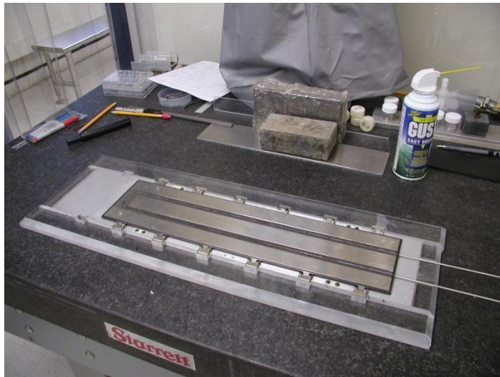
Bottom facing/tube-foam ready for vacuum bagging
