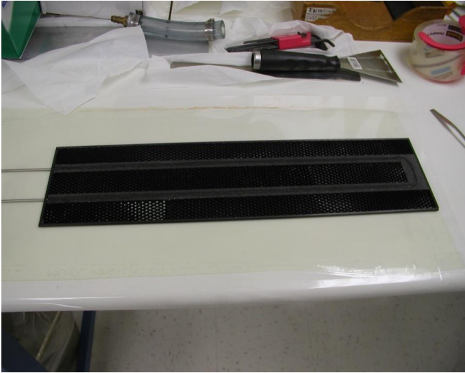
Core prior to 2 nd facing
