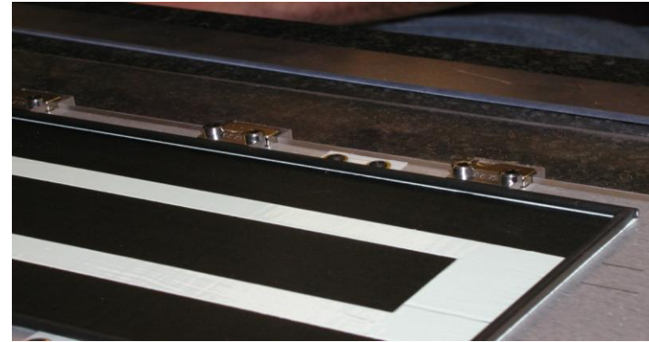
Bottom facing with CF tubes, closeouts and BN loaded Hysol ready for tube-foam subassy.
