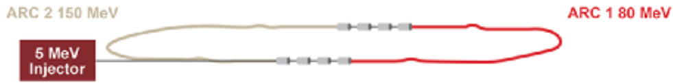
Figure 3.2: The facility is designed in a modular way. This picture shows a Step 1 layout of two parallel cryomodules to achieve \sim 75 MeV acceleration per linac and a final beam energy of 155 MeV (or half of it with just one initial cryomodule).
